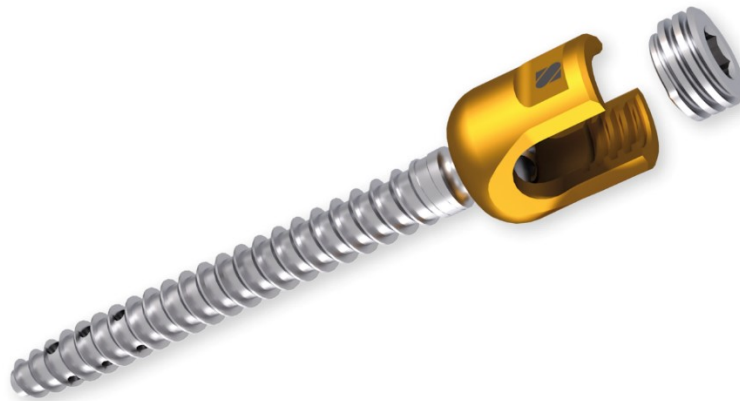
Figure 12: A pedicle screw (MONOPOLY). Cement can be injected into the screw and exits from the holes in the lower part of the screw.
